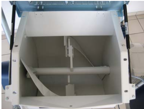
View inside the EMS 60 with exchangeable mixing tools
